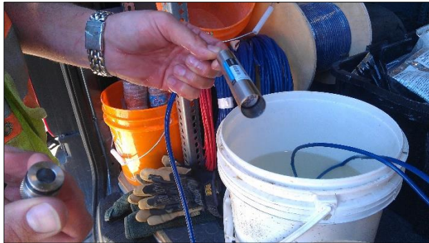
Figure 7. Vibrating Wire piezometer
